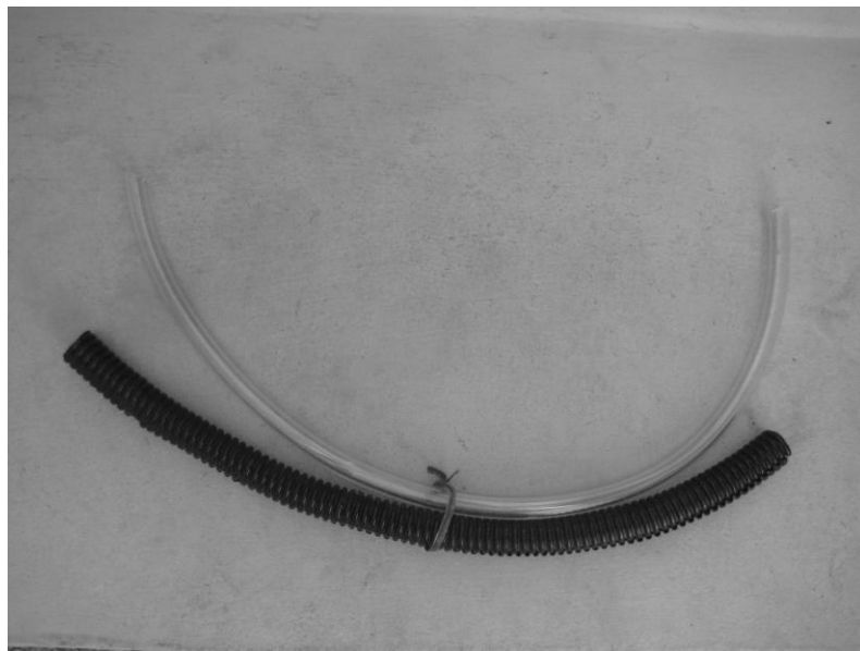
You can use homemade protectors as shown here, or store-bought versions made for managing computer cords.
